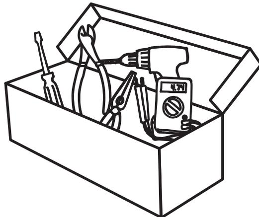
1. screwdriver 2. wire cutter 3. needle nose pliers 4. meter 5. drill
